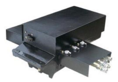
Electric Point Machine (RDL-1) is a non-trainable point machine it is designed to fulfil the strict requirements of safety and reliability for operation of points. It is operated electrically and incorporates an internal point lock and detection mechanism. The machine can be provided with motor to operate on DC or AC, single phase / three phase power supply. In the event of a power failure or emergency the point can be moved to the full normal or reverse position by means of a crank handle.
