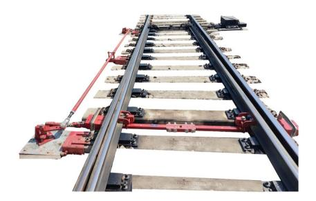
Back Drive system is a mechanical rodding for force transmission, which operates up to two locking positions and ensures min opening and housing at JOH. The compact system is installed at track side and associated lever mechanism is fully covered. This mechanism can be used efficiently for turnout geometries with up to 2 locking levels.
